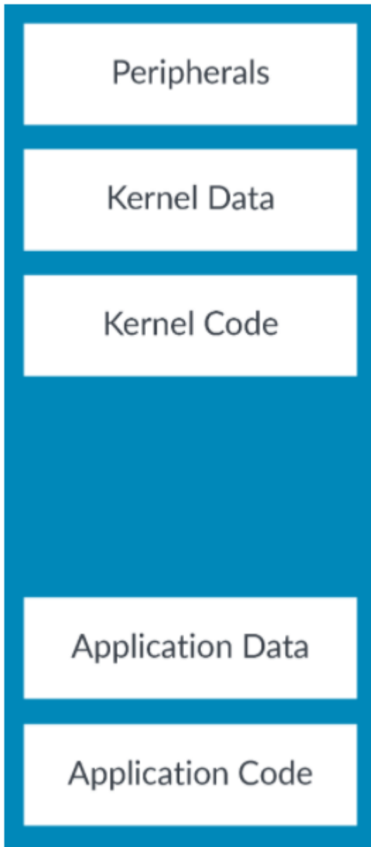
Figure 2-1: A diagram showing simple address space.
